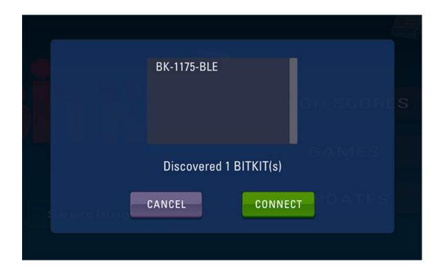
Solid building materials like concrete, brick, and metal, can block or interfere with the Bluetooth signal. This may include the arcade cabinet itself, so try opening the coin door or back door and establish line of sight with the BitKit2.
